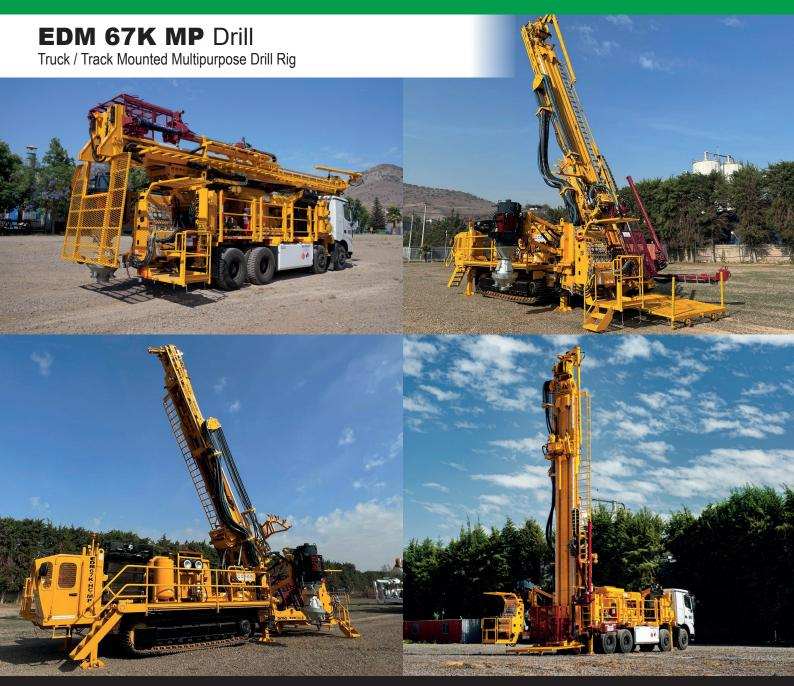
The EDM67K-MP Drill is a heavy-duty multipurpose rig capable of carrying out many different drilling methods in a highly productive and safe manner. The rig features 67,000lbs of pullback capacity, can be track or truck mounted or delivered ready to fit on a customer's own carrier. It can be configured with a Sullair 1350CFM/500PSI compressor onboard, or without a compressor ready to drill with an independent air package.
