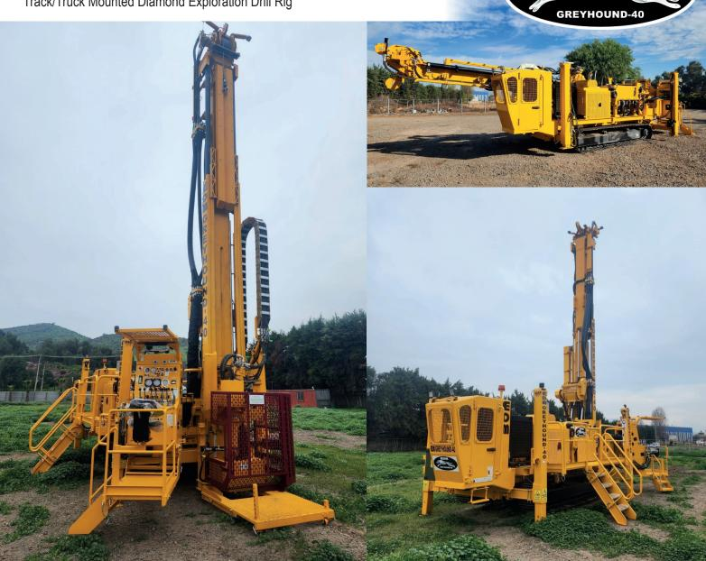
The Greyhound 40 is a high capacity dedicated diamond drill with a compact design offering quick and easy mobilisation and impressive manoeuvrability around sites. With 40,000lb (18,144kgs) pullback capacity, a high-performance top drive rotation head, 40,000lb single line pull main winch and a 260HP engine, the Greyhound 40 offers impressive power and performance for its size.
