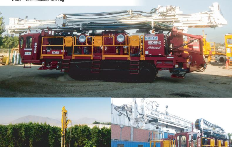
The EDM95K-RC Drill is a heavy duty dedicated reverse-circulation machine built to provide unmatched performance on the deepest and most challenging RC projects in the toughest conditions. The rig has 95,000lbs pullback capacity, can be truck or track mounted and comes with all the safety features required for working on Tier 1 mine sites.
