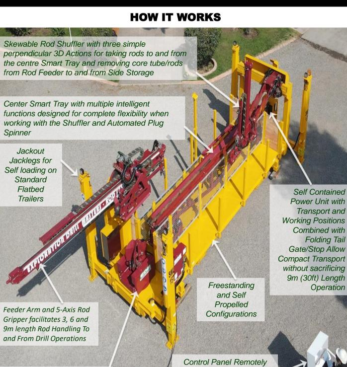
Automated plug assist spinner for inserting/removing haul plug during tripping operations Control Panel Remotely
