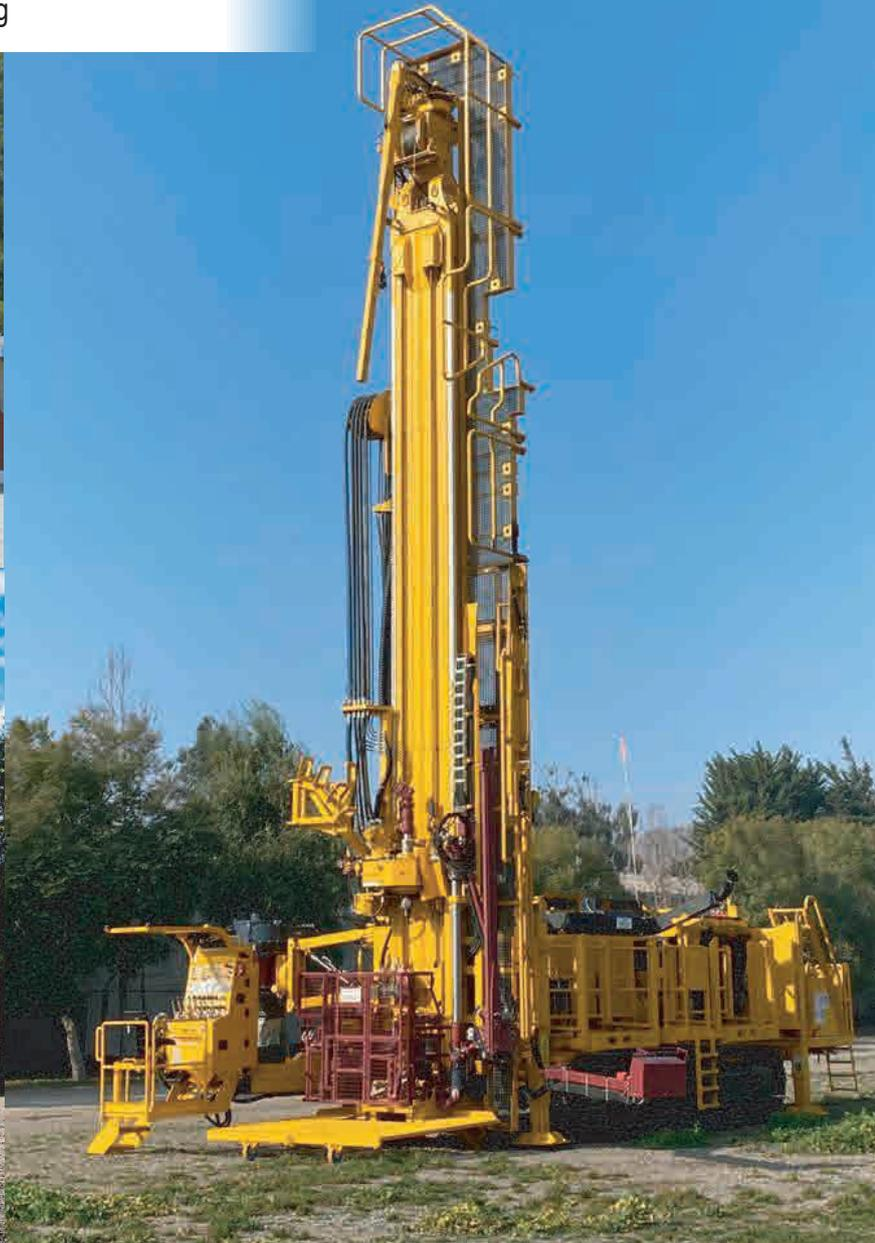
The EDM 67K is a heavy duty drill rig with diamond or multipurpose configurations, truck or track mounted.
