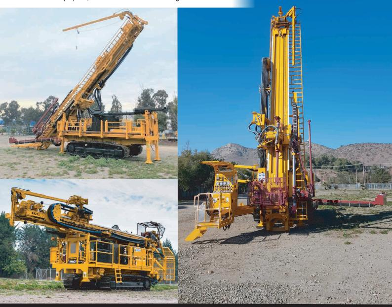
The EDM47K is a light and versatile exploration drill rig with diamond or multipurpose configurations.
