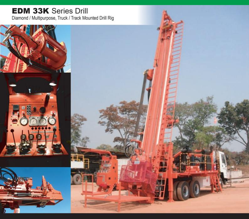
The EDM33K is a light and versatile exploration drill rig with diamond or multipurpose configurations.
