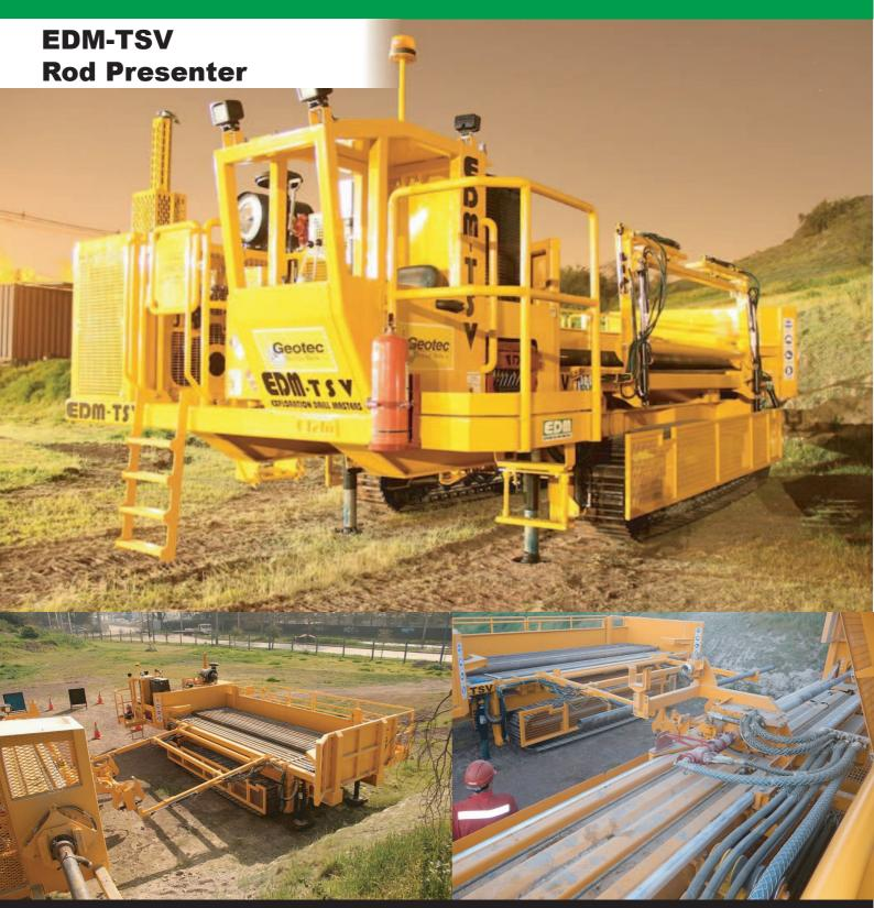
Te EDM-TSV Rod Presenter handles drill rods to and from an EDM horizontal drill mast.
