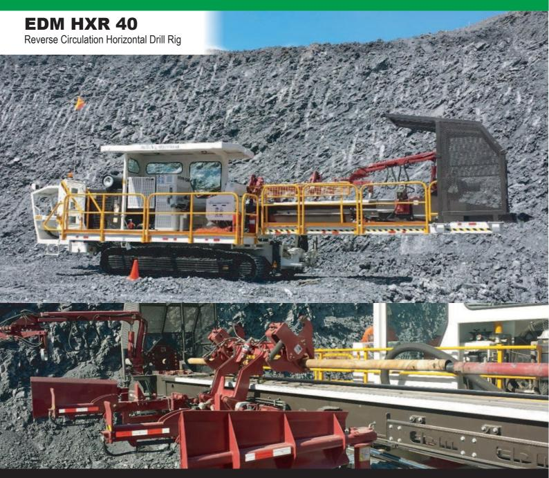
The EDM HXR 40 is a heavy duty and powerful horizontal drill rig that is track mounted and configured for reverse circulation.
