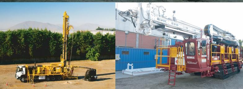
The EDM95K is a heavy duty drill rig with diamond or multipurpose configurations. It can be mounted on self propelled crawler.
