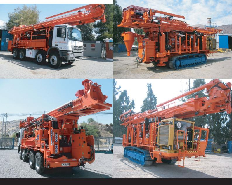
The EDM 67K is a heavy duty drill rig with diamond or multipurpose configurations, truck or track mounted.
