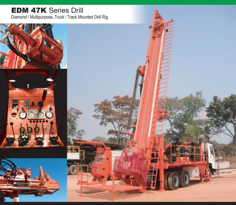
The EDM47K is a light and versatile exploration drill rig with diamond or multipurpose configurations.
